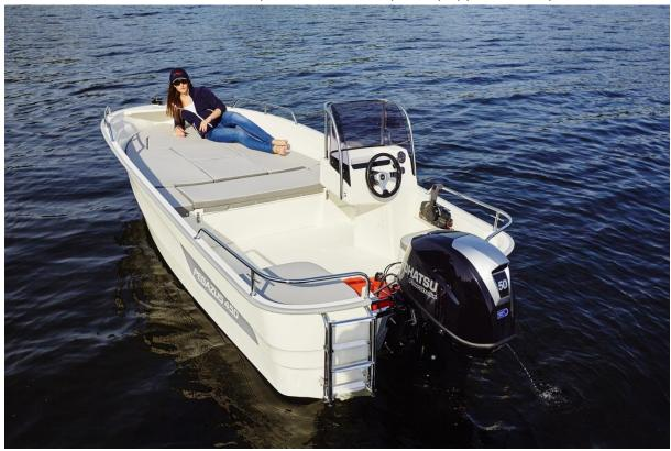
Minimum recommended engine for Pegazus 450 standard version is 15/20HP. Below unit equipped with Suzuki 20HP with low load and 2-3 people on board reached planing speed of around 31 km/h. A very good "price to power" choice is 30HP, especially with tiller steering. If you plan to run the boat with full load and 5 people on board then a 50HP is a safe choice.
