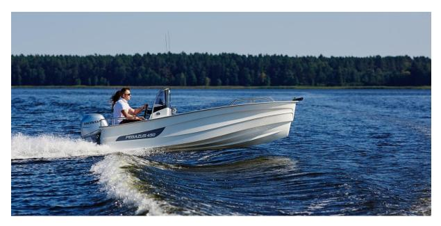
Extended rear on the both sides of the transom create additional rear floatation and work as "trim flaps" so the boat is not afraid of increased weight on the rear, starts faster and the most important – does not lift the bow during drive.
