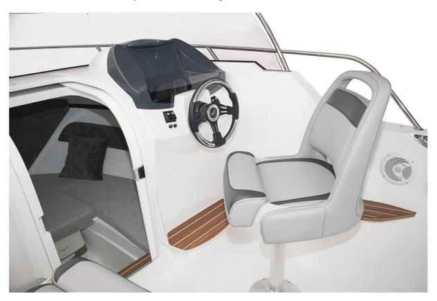
Steering console has a plenty of space for marine equipment and engine gauges. Both steersman's and passenger's seats are turnable and their's front part moves upwards giving support during standing behind a wheel.
